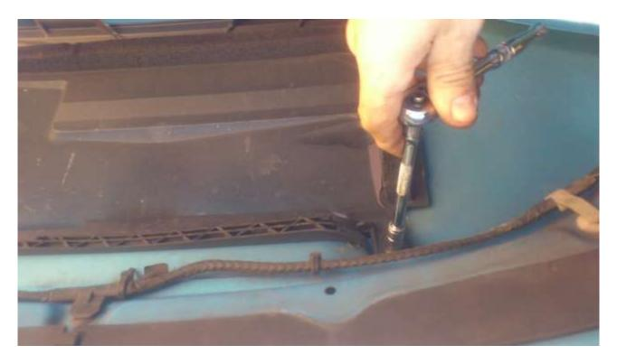
Once the diverter is removed, re-attach the two nuts to hold the air scoop firmly in place.
