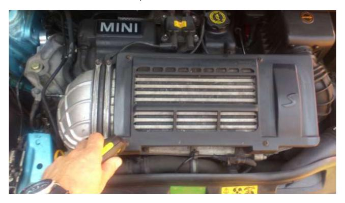
Then remove the stock intercooler air diverter. It may be stuck down with some added rubber pads, gently pull the intercooler away and it will release from the tabs. You will be left with the following -
