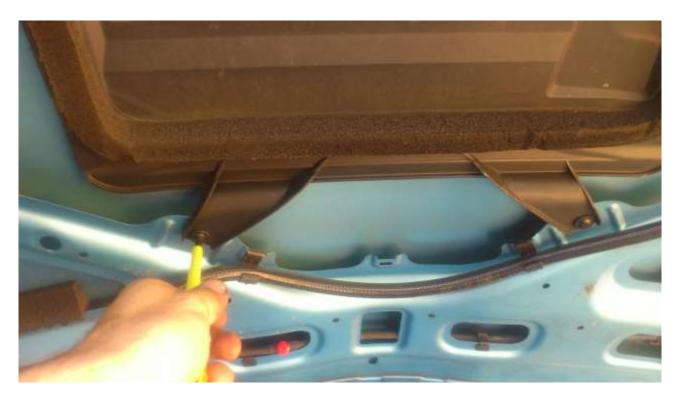
Then undo the two no.8 sized nuts from the underside of the bonnet diverter. These are located next to the scoop entry on the inside of the bonnet. Take care not to force these nuts as they are held in place by small sections of plastic on the underside of the bonnet scoop.
