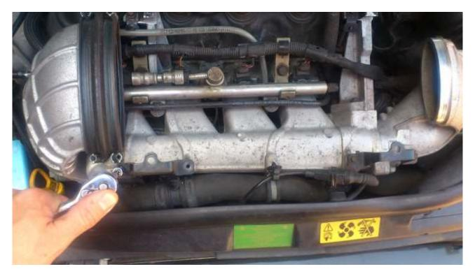
**Step Five**Re-attach the bracket at the front holding the sensor back in place
