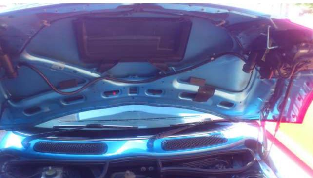
Please note, the removal of the under bonnet insulation is not required to install your Airtec top mount intercooler.
