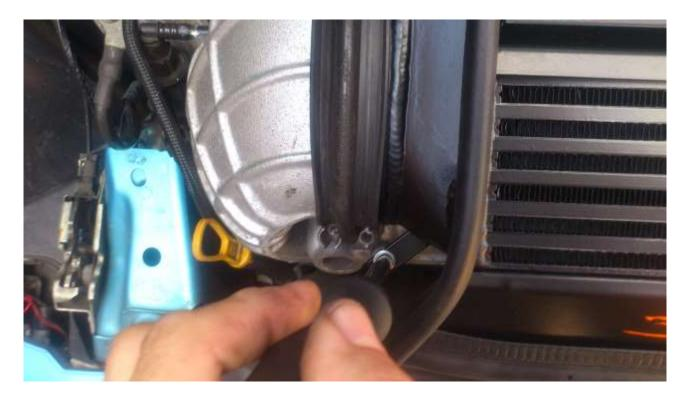
Then re-attach and tighten the clamps on both sides of the intercooler.
